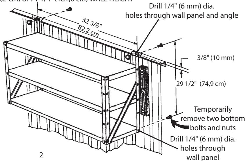
\* Shelf may be attached to horizontal sided buildings if located between wall studs using this procedure.
