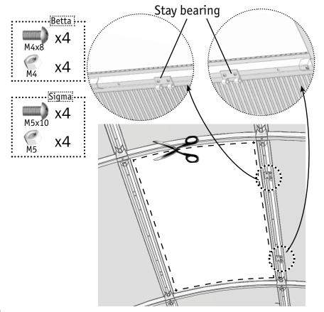
Install the strip on perimeter of the cut of the greenhouse, engaging it on the edge of the polycarbonate. The edges of the weather strip should be expelled out of the cut to drain the rainwater. Cut the hard part of the projecting edge to do it.
