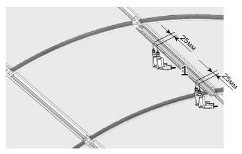
Cut out polycarbonate on as per inner contour of the vent frame. Install the stay bearings in the uppermost bearer.
