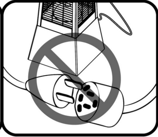
**Caution:** Do NOT use with an extension cord or relocatable power tap (outlet/power strip).
